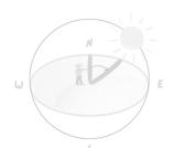
The Azimuth angle is the horizontal angle measured clockwise from North.
